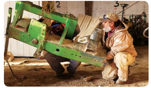
Our Corn Chopper JD 25 decided to give us double trouble. First repair was to the hydraulic system, and then went the PTO. Carlos Aparicio (19 years with JFS) and Aurelio Gonzalez (31 years) have it handled. Chopper is back to work!
