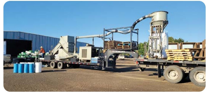
Hosting a pesticide container recycling event was fascinating. Empty, triple-rinsed containers were fed onto the shredder machine, processed and packed into giant sacks for transport.
