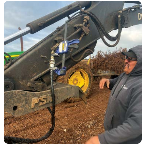
Marco Francisco Gomez shows off a modified clamp that the Hood Acres Machine Shop built for him. Before the disconnect clamp, Marco would have to find a mechanic to bleed the hydraulic pressure off before connecting the grapple. Now he can do it by himself in 5 minutes.
