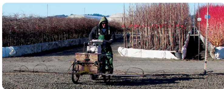
Augustin Moo using his custom line painting bike on the gravel at CF. Augustin carefully reads set off orders that Martin Nunez produces to mark out line spacing for new potting. Because of how like trees are grouped together there are often a lot of line changes within the same bin.
